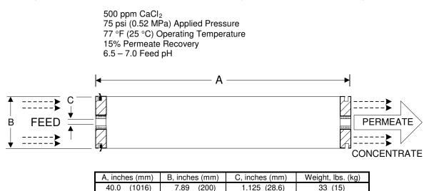
Notice: Permeate flow for individual elements may vary -20/+25 percent. Membrane active area may vary +/-4%. Element weight may vary. All membrane elements are supplied with a brine seal, interconnector, and o-rings. Elements are enclosed in a sealed polyethylene bag containing less than 1.0% sodium meta-bisulfite solution, and then packaged in a cardboard box.
